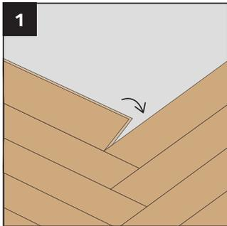
Each board needs to be locked into one another. To connect a new board you have to use a rubber mallet to gently engage the locking system.
