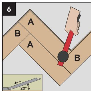
As done with the first 2 boards, use the soft rubber mallet to gently tap down on your boards to ensure the locking system is in the correct place.
