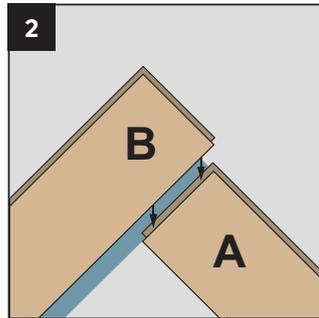
Position the long side of plank "B" over the short side of plank "A", so that the flooring can fit together without any gaps.
