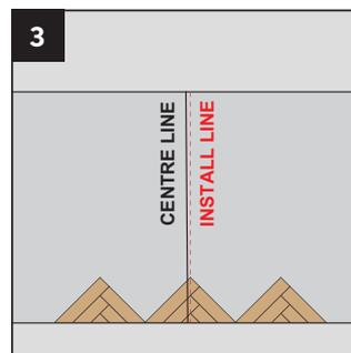
Lay out your starting triangles along the wall which you are installing from. Start by placing the point of your first triangle pointing up your installation line. Place your 6mm spacer behind the triangles to ensure the necessary expansion is left. Lay the rest of your triangles across the width of your starting wall with expansions behind each triangle.
