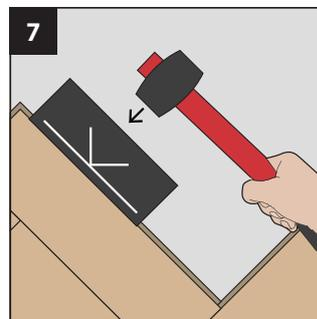
Use a tapping block along the long edge to close any small gaps between the rows. Tap gently to avoid damaging the product, this could impact on your installation.
