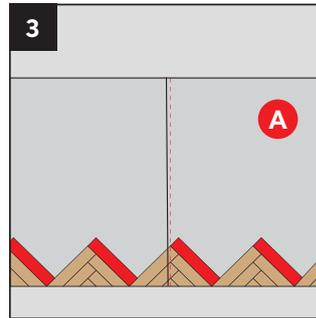
To connect your triangles together into one piece, start by installing A boards as above. It is important to install these boards first and check all edges to ensure they are connecting the floor together correctly. Cut any "A" board to size that might be against a wall and installing your 6mm perimeter spacers as you progress.
