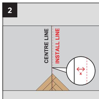
Mark the installation line on your sub-floor parallel to the center line as shown above. This should be at your X distance away from the center line.
