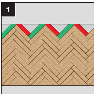
The alternating installation of "A" boards followed by "B" boards per row continues. However, you will need to start cutting boards to size to finish your installation. When cutting boards to size you must ensure you leave the correct gap for your spacers, keeping your expansion gap uniform around the full perimeter of your room.
