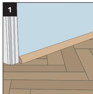
Once the floor is installed, remove the spacers; sweep the floor with a soft brush. Fix the skirting/base boards or suitable edge trim (available from your local distributor) to cover the expansion gaps. These should be attached to the wall, not the floor. This will allow your product to remain free to expand underneath the trim.
