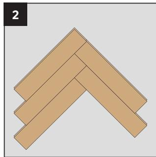
Install your "A" and "B" boards together as shown above. You must ensure no gapping between the joints is present. Refer to section A of these instructions as guidance should it be required.
