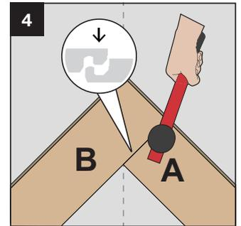
Using a soft rubber mallet, tap down gently on the joint between both boards. This will make sure your flooring is locked into place. The groove side of your planks must always face away from your starting wall.
