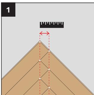
Measure the distance between the corners of your flooring, as shown on the picture above. Divide this number by 2, this will provide you with your installation value known as X.
