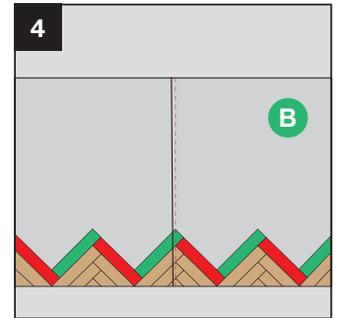
You can now install your "B" boards as shown above into your previously installed "A" boards. It is important after every row has been installed to check your flooring is running parallel to your installation wall, following the installation line. You might have to adjust as you go to ensure straightness is achieved.
