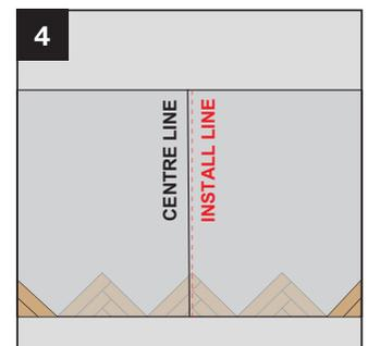
To finish your starting rows, measure the gap between your wall (including Spacer) and closest installed triangle. Mark this distance onto one of your triangles. Cut to size and position in place.
