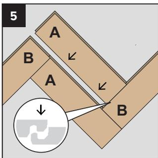
Take your next "A" board and insert the long tongue side into the previously installed "A" & "B" boards. Make sure your "A" board also overlaps the other "B" board perfectly so all joints are aligned.
