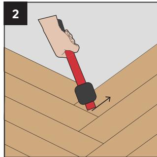
Using your rubber mallet gently tap down on each board during installation to connect the short side into the previous board. Start in the corner and work towards the opposite short side edge. A tapping block can also be used if required to close up slight gaps in the joins.
