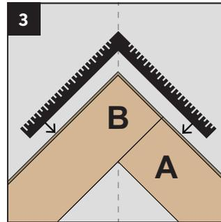
To ensure your boards are perfectly aligned at a 90\* angle, we recommend using a set square when putting the first 2 rows together. It is critical to ensure you install your first few rows correctly for a successful installation.
