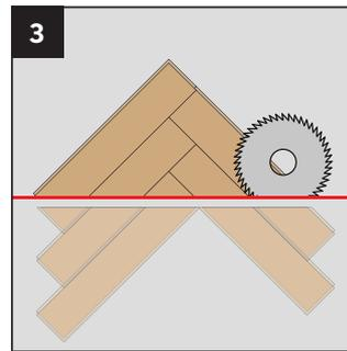
Use a straight edge to mark a line going across your flooring as shown above. This will create your triangle to start your installation. Depending on the type of saw you use, it might be easier to disassemble your flooring to start your installation. Do not throw away your waste, this can be used later in the installation.
